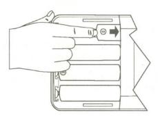
**Note:** Be sure to insert each battery with the proper polarity, as marked in the battery compartment.
